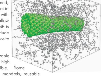
SMP currently functions on thermal activation customizable from -30°C to 260°C (-20°F to 500°F). Extremely high temperatures and cryogenic ranges may be possible. Some examples of applications include custom reusable mandrels, reusable molds, replica optics, and deployment mechanisms for outer space.
